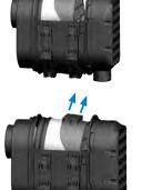
**Remove primary filter.** Pull the filter out of housing. For side service access models: you must first loosen the filter gasket seal. Using the handle, push down on the filter to loosen the seal, which will tilt the filter to approximately a 5° angle.
